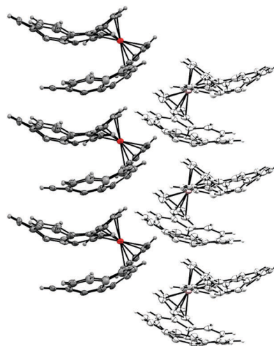
Fig. 4 Stacking motif of 4 between four molecules. View along the crystallographic b -axis. Molecules I: light grey, molecules II: dark grey, the Fe atoms are marked in red.
